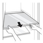
Pinch the sides to open the water filter cover.
