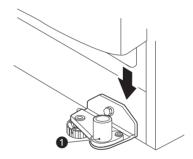
Fit the hinge 2 over the hinge lever latch 3 and slot it into place. Rotate the lever 4 counterclockwise to secure the hinge.
