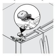
5. Pull up on the water line gently to remove it from the door.
