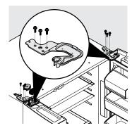
You may need to remove the lower hinges for clearance purposes. To gain access to the lower hinge, first extend the Custom Flex Temp Drawer. Unscrew the 3 lower hinge screws and slide the hinge inward.
