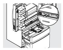
4. Reattach the electrical harness by positioning the cable clips over the black markings on the harness and push the 4 cable clips through the openings in the rail to secure the harness in place.
