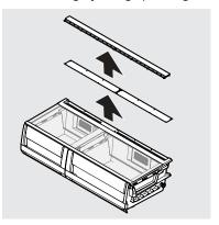
Removing Auto Humidity **Control Membrane**
