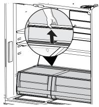
Removing Auto Humidity Control Membrane
