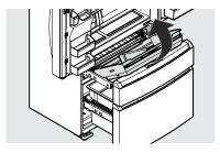
Unsnap the 4 cable ties by pressing clip sides together and pushing them through the opening.
