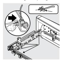
4. Remove the screw and the retaining clip and disconnect the harness.
