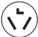
3-wire receptacle (10-30R)
