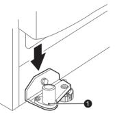
Fit the hinge Over the hinge lever latch and slot it into place. Rotate the lever Clockwise and fasten the hinge.
