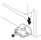
2 Fit the hinge 2 over the hinge lever latch 3 and slot it into place. Rotate the lever 4 counterclockwise to secure the hinge.
