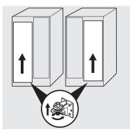
After leveling, verify the door stop contacts the lower hinge and the top of the door does not contact the upper hinge through full movement of the door (from fully closed to fully open).
